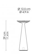
A rechargeable table lamp with painted aluminium fixture, a polycarbonate diffuser and a LED light source. Painted aluminium fixture. Lightweight and practical, it is ideal for use in any context and surroundings. Its IP54 protection rating makes it ideal for indoor and outdoor use. Dama comes in two colours: matt white or black. Version with a USB port at the side for charging mobile devices, The battery has a life of 9 hours, unless the charging mobile devices function is used
